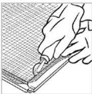
around the frame. *If applying to a wooden frame:* secure screen using nails or heavy duty staples at 0.3 – 0.5ft (10-15 cm) spacing. *If applying to a metal or vinyl frame:* lay the spline
