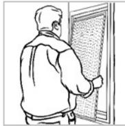
2. **Unpack the PermaNet® Screen fabric** Using scissors or a utility knife, cut the screen 1 inch larger and wider than the frame on all sides.
